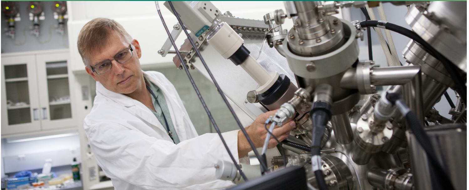
John Baltrus uses X-ray photoelectron spectroscopy to analyze a material's surface chemistry.
