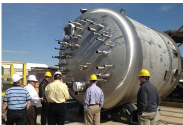
NETL's experimental vessel was designed based on this full-sized vessel at Hanford.
